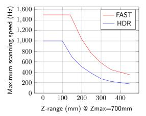
Figure 4: Maximum scanning speed, object far from scanner
