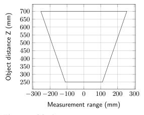
Figure 3: Maximum measurement range
